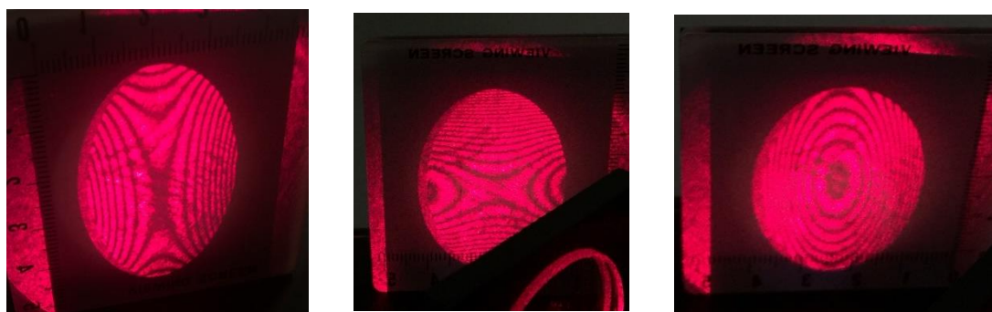
Fig. 9. Interference patterns of different optical path lengths
